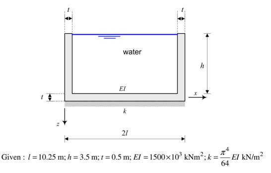
Figure 4 : Aqueduct on an elastic foundation
