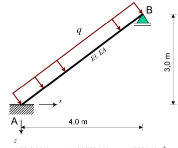
Given : q = 80.8 kN/m; EA = 27000 kN;  $EI = 4000 \text{ kNm}^2$
