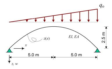
Given : l = 10 m; f = 2.5 m;  $q_o = 50 \text{ kN/m}$ ;  $EI = 25000 \text{ kNm}^2$
