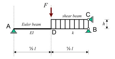
Given : l = 8 m; h = 0.8 m; F = 22 kN; k = 1000 kN; EI = 6400 kNm<sup>2</sup>
