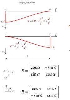
$$\overline{f} = R \quad f \quad \text{and} \quad f = R^T \overline{f}$$
