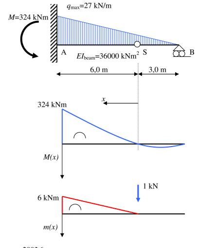
$$w = \frac{1}{EI} \int_{0}^{6} (-x) \times (-9x - 4,5x^{2} - 0,5x^{3}) dx = \frac{2883,6}{EI} = 80,1 \text{ mm}$$
