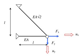
a) If the forces are only applied at the bar ends of the prismatic truss elements, prove the stored strain energy as a result of the  $\Delta l$  equals to:
