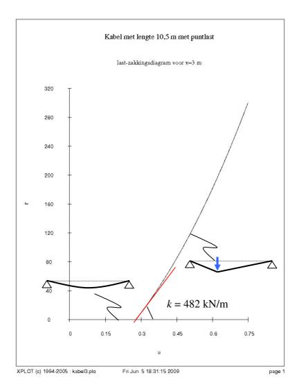
From the graph it becomes clear that the unloaded structure has no stiffness. The shape of the cable first has to change from the parabolic shape in to the bi-linear shape which belongs to the concentrated loading. Starting from 0,27 m the system develops stiffness (with respect to the initial parabola). The slope of the diagram equals to the stiffness and a value of 482 kN/m is found which is slightly larger than the predicted value.
