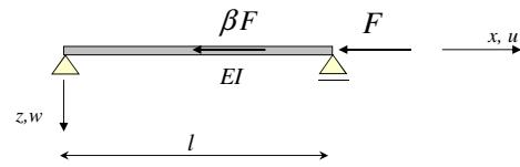
Compressive element with additional loading at mid span
