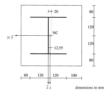
Chose a  $\overline{y} - \overline{z}$  - coordinate system through the normal force centre of the steel section. The normal force centre NC of the entire cross section must be located at the line of symmetry (which is the  $\overline{y}$  - axis, thus  $\overline{z}_{NC} = 0$ ).
