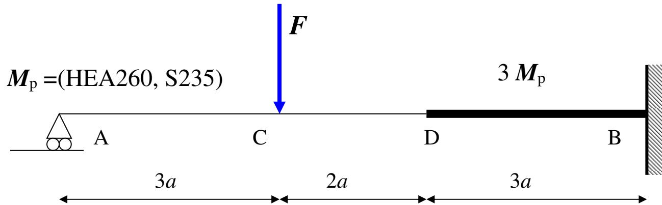
FIND THE LIMIT LOAD or COLLAPSE LOAD  $F_p$  ?
