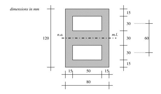
$$I_{zz} = \frac{1}{12} \times 80 \times 120^3 - 2 \times \frac{1}{12} \times 50 \times 30^3 - 2 \times 50 \times 30 \times 30^2$$
