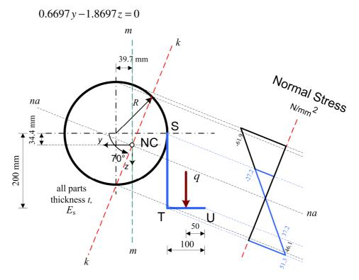
Resulting k-k, m-m and n.a. due to given loads and normal stress distribution
