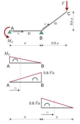
The moment distribution for beam AB and BC with local axis along the beam axis results in:
